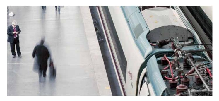
The metal-oxide surge arresters produced by ABB Switzerland Ltd. for DC traction systems are developed and type tested according to the new European standard EN 50526-1 which is specifically for metal-oxide surge arrester in railway application up to 3kV nominal voltage. The surge arresters also meet the requirements for A1/A2 functionality according to VDV 525 recommendation.
