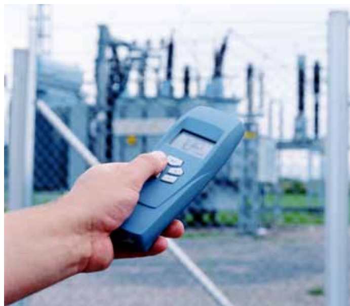
Remote reading with EXCOUNT-II
